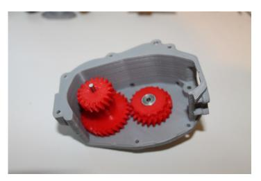
Insert the input shaft into Low Range Gear 1. Shaft should only be inserted into the plastic section. It should not protrude into the bearing. Tighten set screws.
