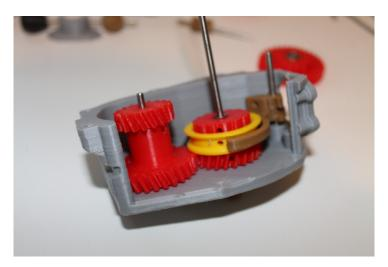
Insert Low Range Shift Collar into Low Range Shift Fork. Install, making sure to align set screw holes on the Low Range Shift Collar to the Low Range Shift Collar Gear. Low Range Shift Collar should spin freely inside Low Range Shift Fork .
