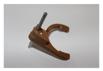
Insert Low Range Shift Rail into Low Range Shifter Fork, Shaft should protrude roughly 0.79" from surface shown.
