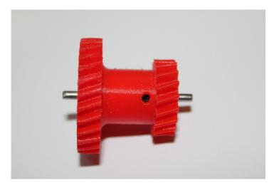
Glue the Low Range Gear Counter Shaft 1 and Low Range Gear Counter Shaft 2, using the Low Range Counter Shaft to align the them. Tighten set screws.
