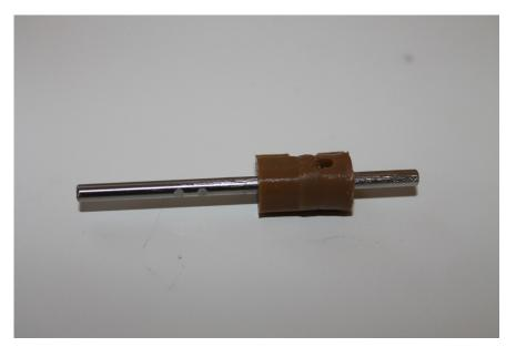
Using sand paper or a file, roughen up the 4WD shift rail. Using super glue install 4wd selector onto the 4WD shift rail. Shift rail should protrude 0.45" on the right side. Refer to picture above.
