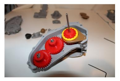
Slide Transfer Case Shift Collar Gear onto output shaft. Assemble 4WD shift collar onto 4WD Shift Fork and slide onto shift rail.
