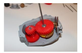
Slide Low Range Gear 2 onto output shaft. Install 4WD shift
