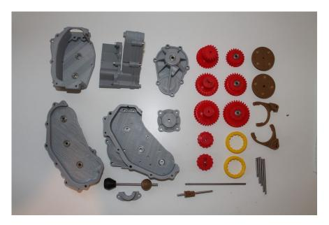
Prepare individual pieces after printing. When reaming holes for bearings and shafts, make sure to keep the hole as concentric and straight as possible. This will eliminate any wobble of the gears while in operation. Keep all holes for shafts as small as possible. You want the 3mm shaft to fit tightly but not too tight to where you can't pull it out by hand.
