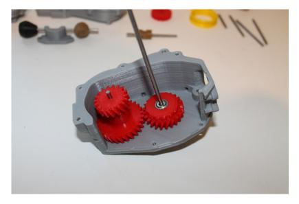
Insert 4WD output Shaft into Low Range Gear.
