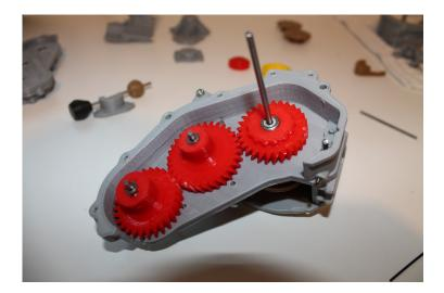
Install 4WD output Shaft into 4wd Final Gear. Install 4WD idler shaft into 4wd Idler. Slide 3WD Gear onto output shaft.
