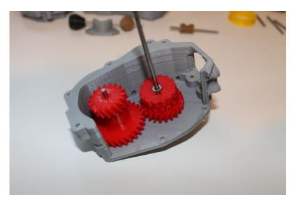
Slide on Low Range Shift Collar Gear, tighten set screws.
